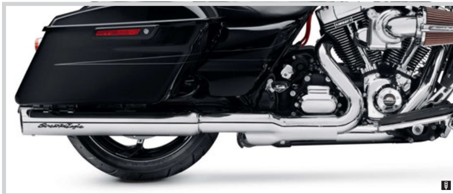
C. SCREAMIN' EAGLE HIGH-FLOW EXHAUST SYSTEM WITH STREET CANNON MUFFLERS – CHROME (SHOWN WITH SHORT SLASH OUT END CAPS)
